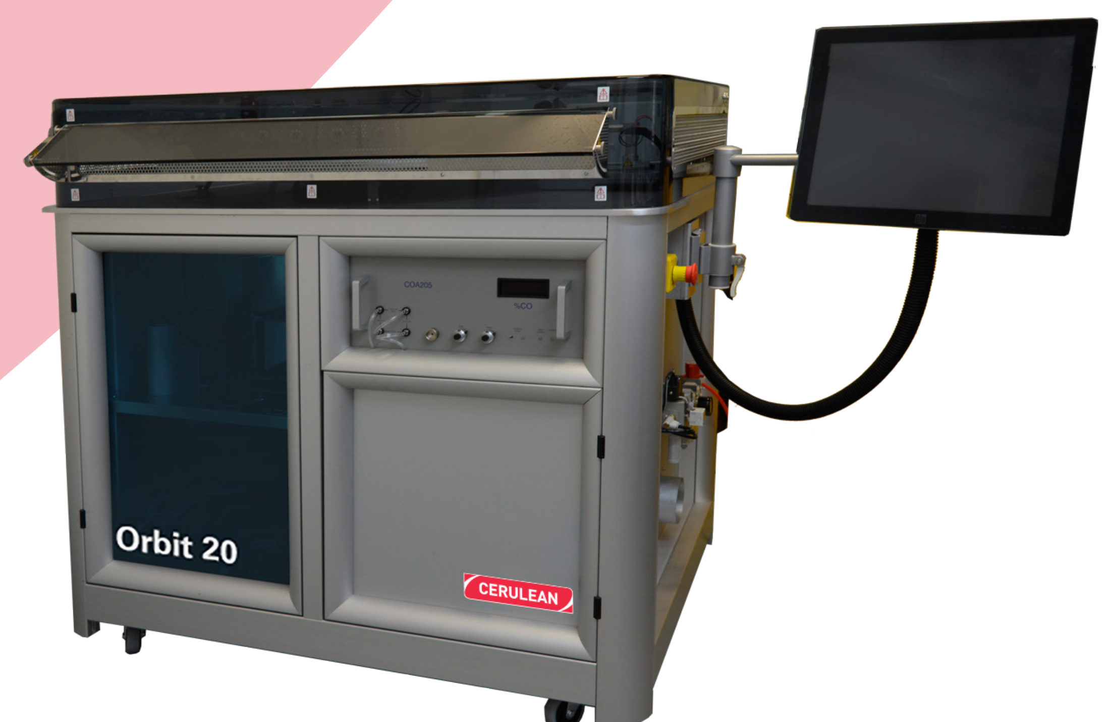
Fig 2 : ORBIT20 and improved low yield loss rotary smoking machine
