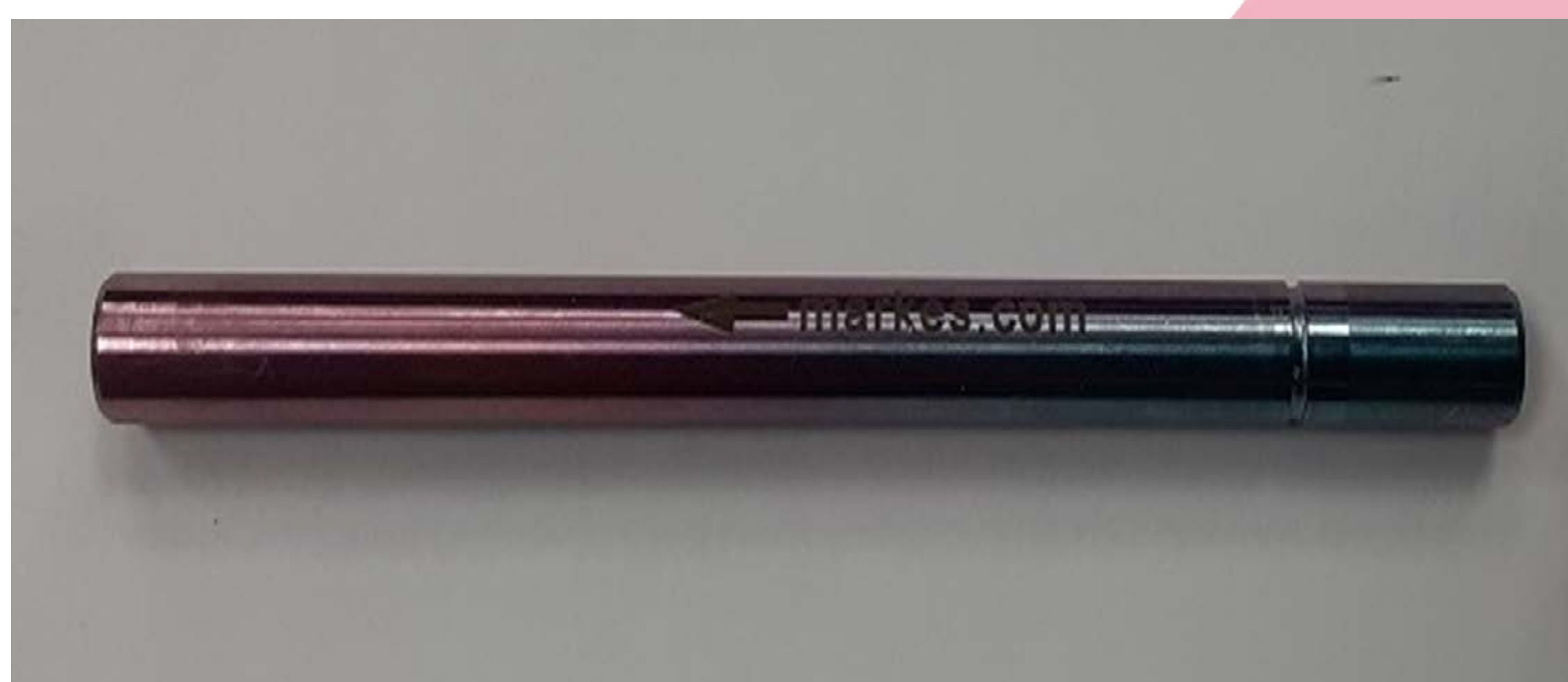
Figure 2: Markes sorption tube used in experiments
