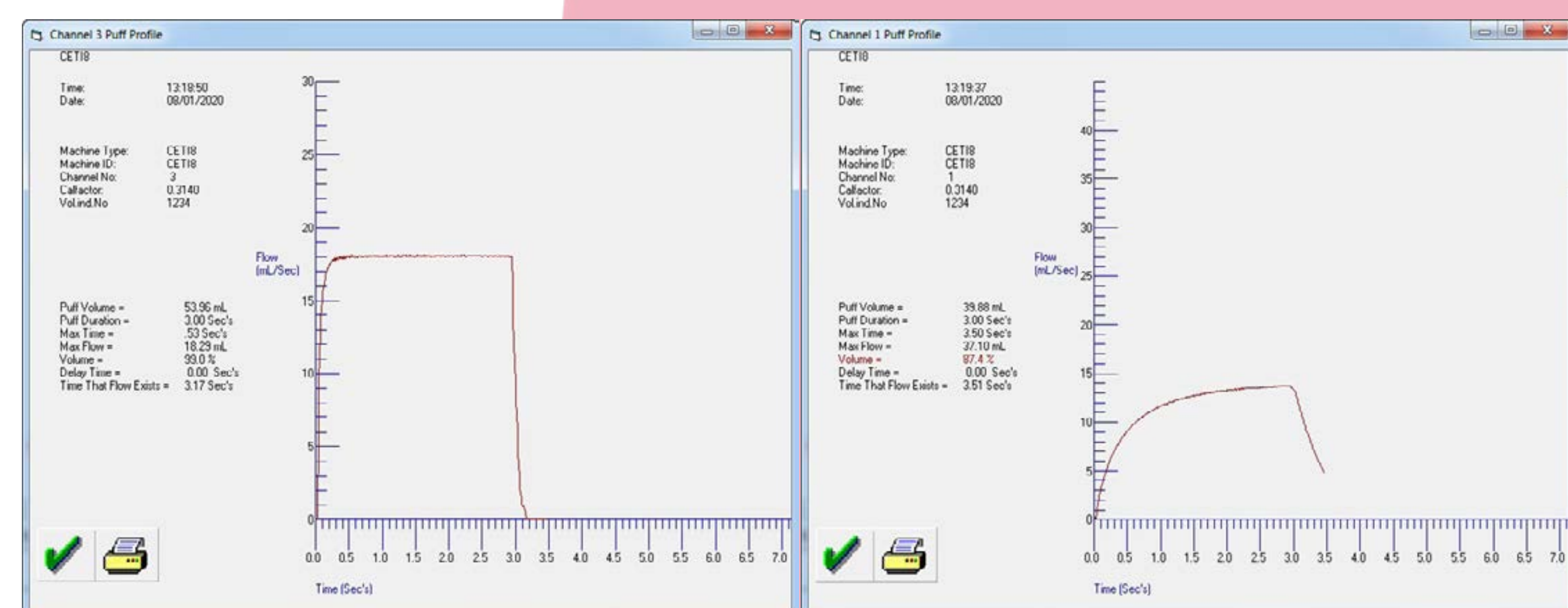
Figure 3: Visualisation of flow, time and swept volume of the CET18 with a 100mmWG pressure drop and Markes TD tube in series. Nominal volume 55ml, puff duration 3 seconds. Measurements made with Cerulean's VFA450RH.
