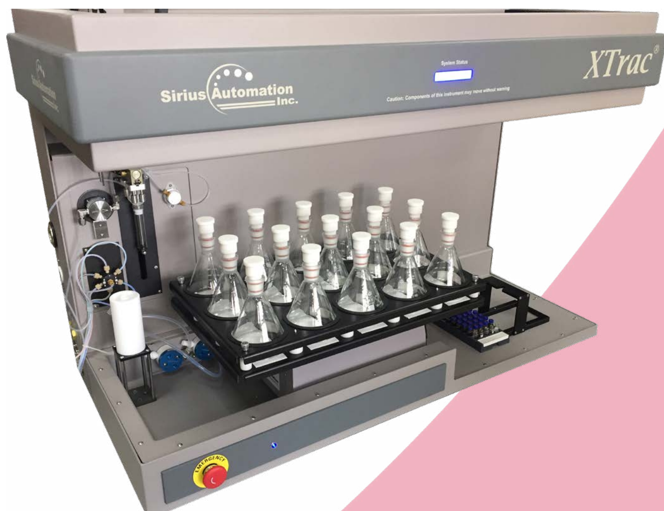
Figure 1: Sirius Automation Xtrac® machine configured for extraction of Cambridge filter pads and dispensing into vials for GC analysis
