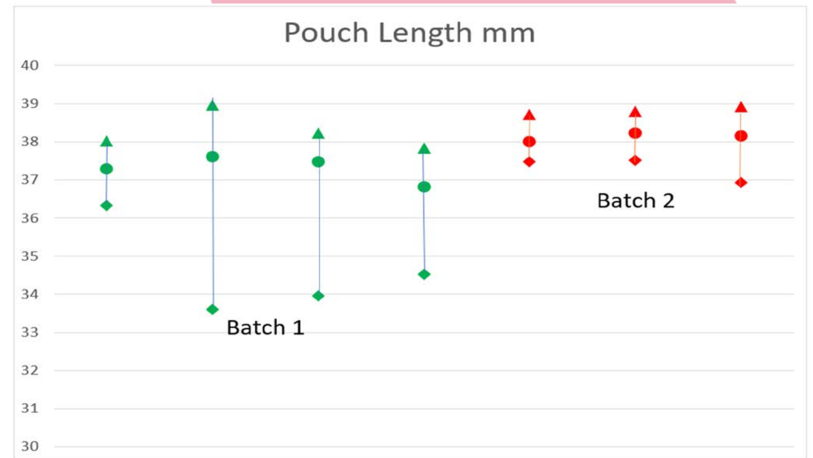
Figure 3: Variation in pouch length for two batches of nominally the same product
