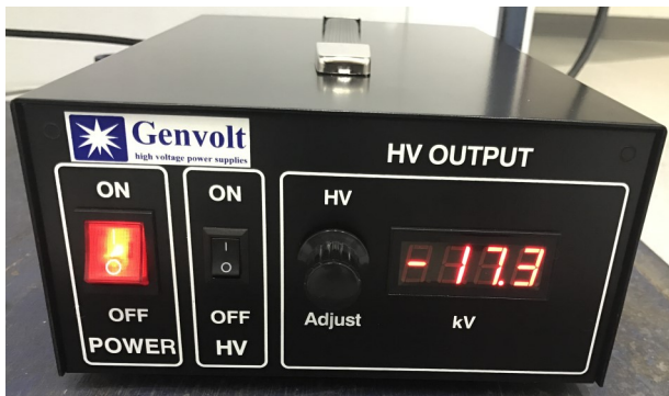
2 x High voltage power supplies
