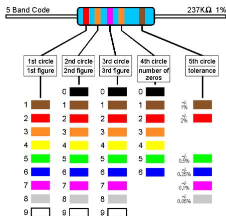
**Note:** The colour of the fifth band from the left (tolerance band) is not important, as close tolerance resistors are not required in this situation.
