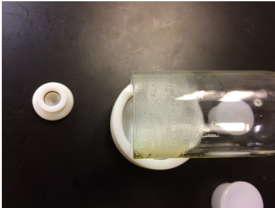
Figure 6: Deposit of cannabinoid oil inside of the Electrostatic trap after 60 puffs of Berry Gelato vapour. Experimental conditions 55/3/30 and 20kV on electrode.
