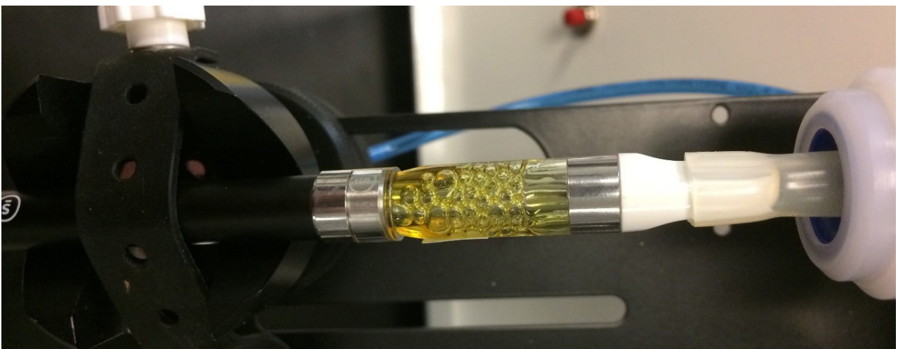
Figure 4: Cannabis vape cartridge showing "frozen" liquid bubbles within the cartridge. Returning the cartridge to an oven for 30 minutes restored some fluidity to the liquid although not all bubbles disappeared.
