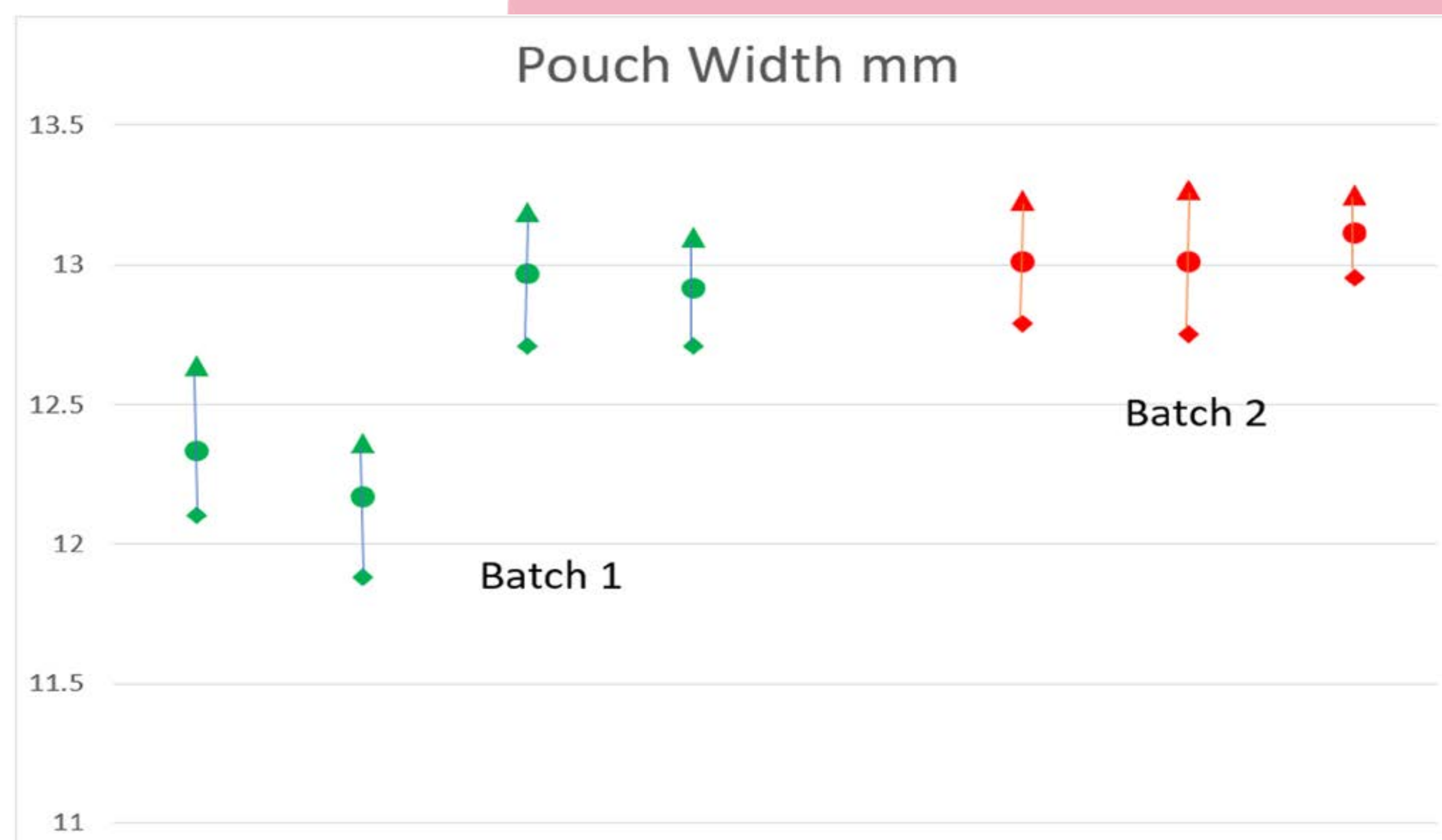
Figure 4: Variation in pouch width for two batches of nominally the same product
