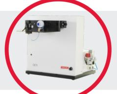
The **Aura** is an entry level 5 port Continuous Aerosol Generator (CAG) for testing electronic cigarettes/vape, cannabis vapes, or HTP devices. It allows the user to program a puffing regime. The user can select puff shape, volume, duration, interval, and overlap period to deliver a continuous aerosol for analysis or exposure. Angled vaping is standard on the Aura.
