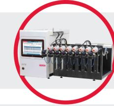
The **CETI8** is an eight port machine for testing between one and eight devices and is fully compliant with ISO20768:2018. The CETI8 allows the user to program a puffing regime for establishing delivery from various e-cigarette devices.
