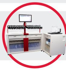
The **CETI20** is a next generation 20-channel analytical linear Vaping machine dedicated for testing e-cigarettes and Heated Tobacco Products (HTPs). This machine is equipped with twenty 210ml intelligent puff engines, new beckhoff control system and intuitive user interface (UI), vaping bar angle feedback, button activation and battery charging module.
