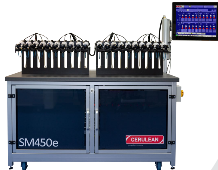
Cerulean SM450e with integrated temperature sensors
