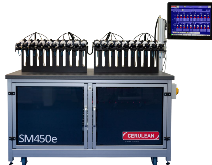
Cerulean SM450e with integrated in-line CO Sensors
